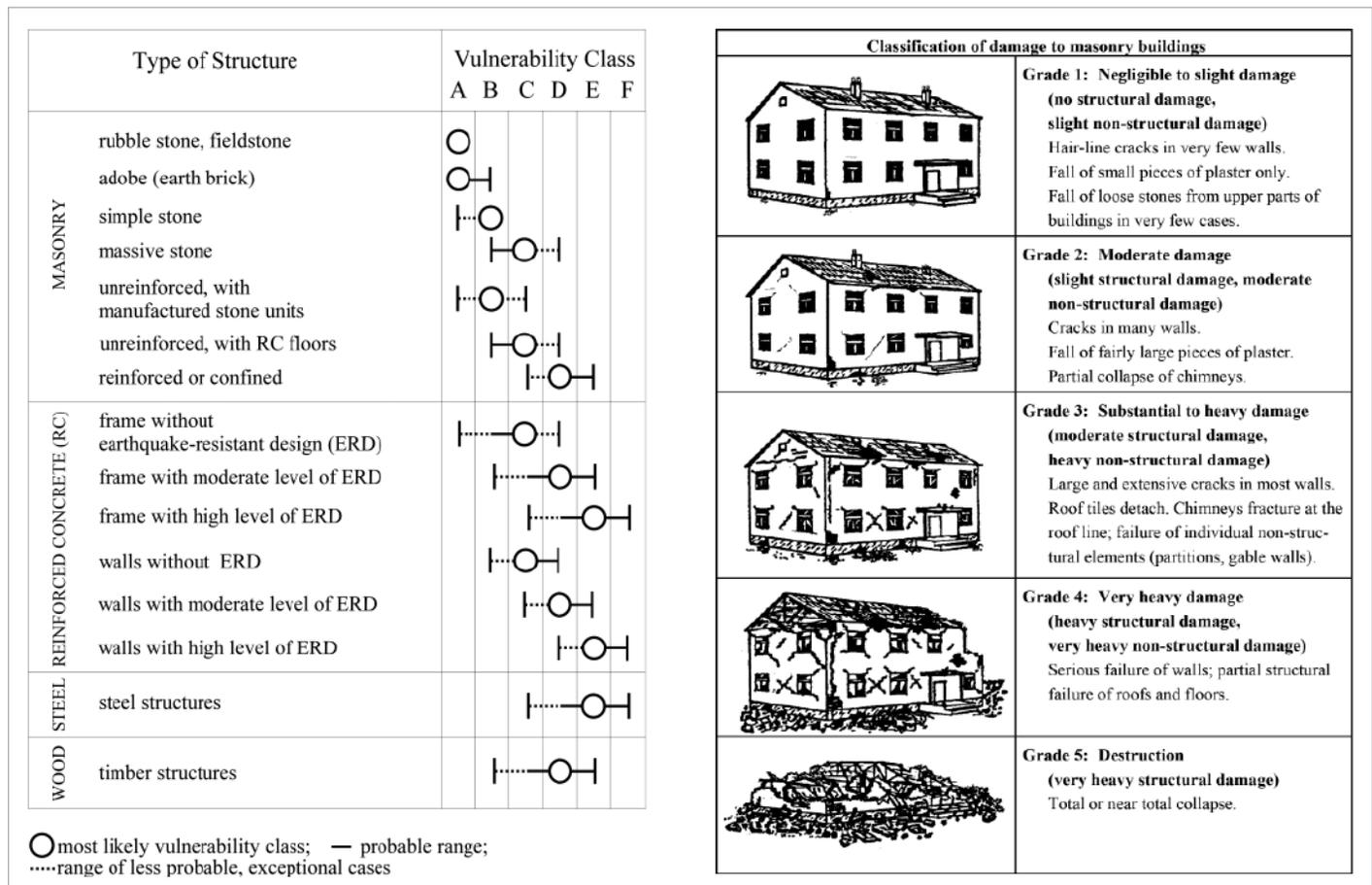
Fig. 2. The European Macroseismic Scale defines vulnerability classes for different building types (left) as well as damage grades for building types, including masonry buildings (right). Credit: Grünthal [1998]
