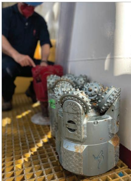
The JOIDES Resolution crew used rotary drill bits to extract the core from the seafloor. Credit: Sarah Treadwell, Communications Officer, IODP Expedition 399
