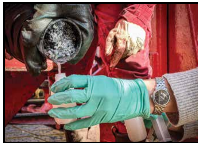
Susan Lang takes a water sample directly from the core liner on the rig floor. Credit: Erick Bravo, IODP JRSO, CC BY 4.0 ( bit.ly/ccby4-0 )
