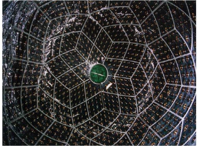
The Kamioka Liquid Scintillator Antineutrino Detector can ascertain the presence of electron antineutrinos produced through the decay of uranium and thorium deep inside Earth when they collide with atomic nuclei. Credit: Research Center for Neutrino Science, Tohoku University
