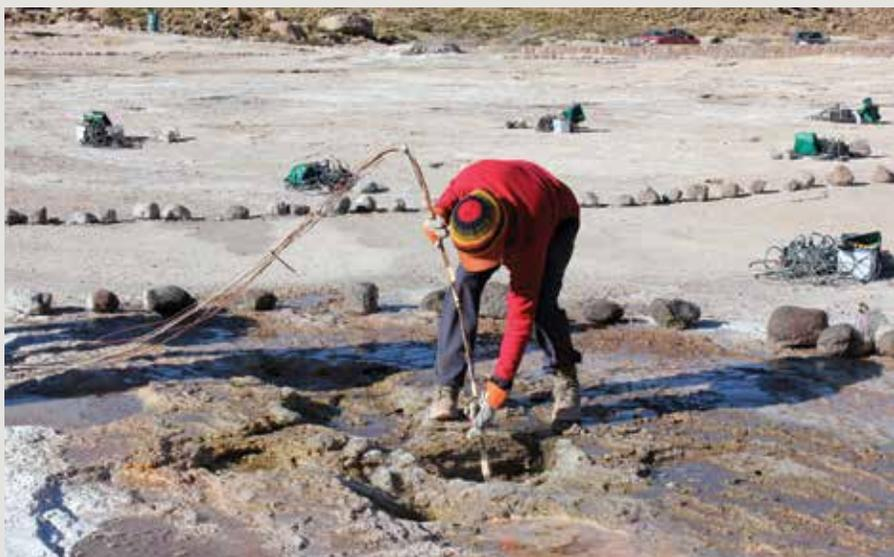
Carolina Muñoz-Saez inserts pressure and temperature sensors into a geyser conduit at El Tatio in northern Chile. Seismometers that measured seismic tremor throughout many eruption cycles are visible in the background. These experiments were conducted in coordination with the communities of Caspana and Toconce. Credit: Max Rudolph, University of California, Davis
