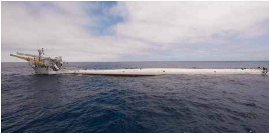
FLIP lies in its horizontal position as it is towed to a research location off the coast of California. Credit: John F. Williams/U.S. Navy, CC BY 2.0 ([bit.ly/ccby2-0](http://bit.ly/ccby2-0))
