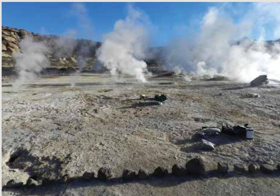
An array of instruments (foreground) measures seismic tremor around geysers at El Tatio in Chile. Credit: Shaull Hurwitz, U.S. Geological Survey
