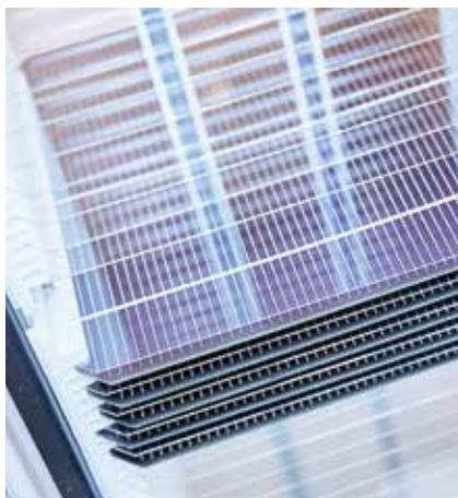
Perovskite-silicon solar cells set a record solar cell efficiency of nearly 30%. Credit: Oxford PV
