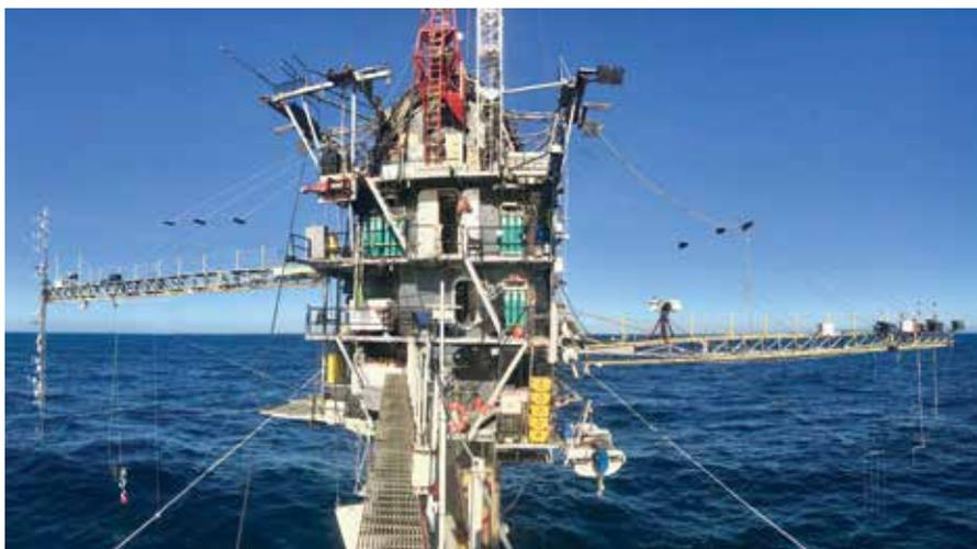
*FLIP* is a very large spar buoy: It sits upright at the ocean surface and is specifically designed to respond minimally to surface wave motions. The author took this photo of *FLIP*'s "face" during the 2017 CASPER field study from the end of one of the platform's three foldable booms, aptly named Face Boom. Credit: David G. Ortiz-Suslow
