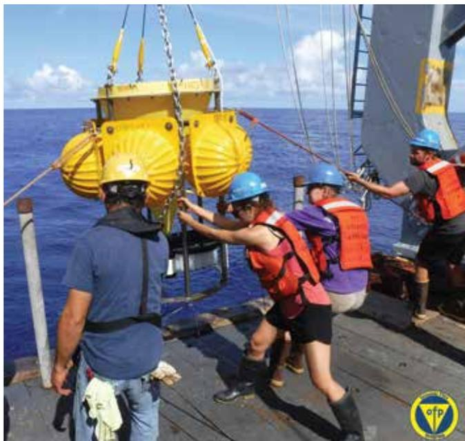
An Oceanic Flux Program time series sediment trap deployed at 3,200-meter depth comes on board R/V Atlantic Explorer. Credit: J. C. Weber
