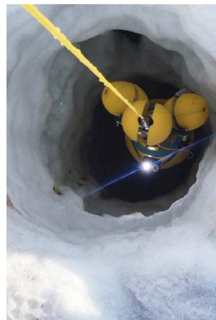
*Icefin was pulled back up to the surface through a borehole drilled into Thwaites Glacier. Credit: Icefin/ITGC/Schmidt*
