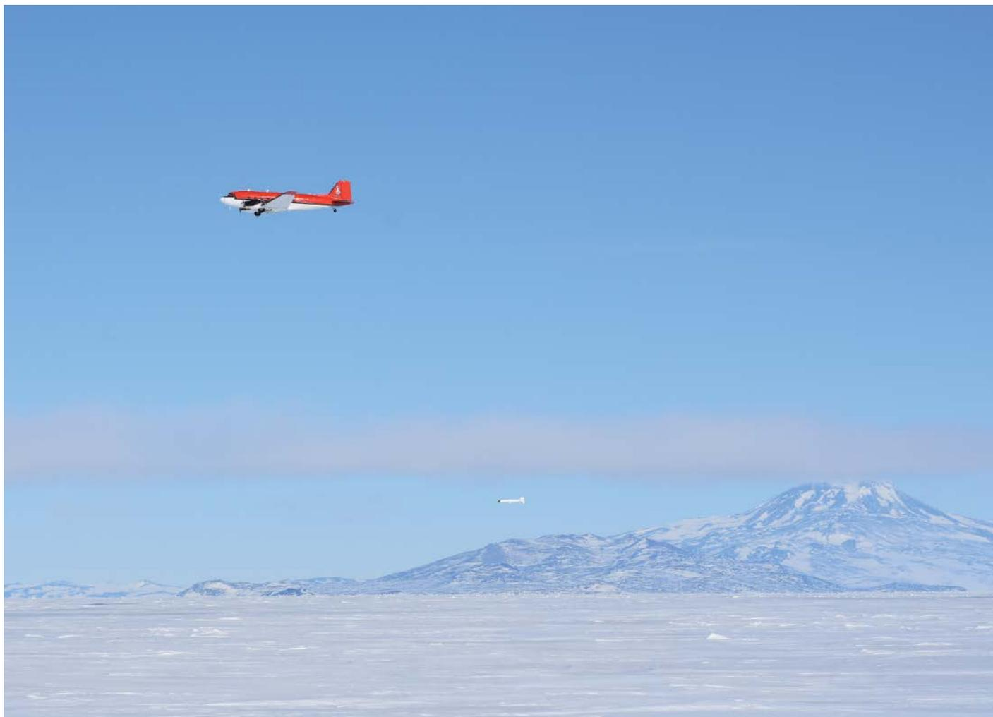
An aircraft tows the electromagnetic induction bird (visible at the center) over fast ice in McMurdo Sound, Ross Sea, Antarctica. Credit: Greg Leonard, University of Otago
