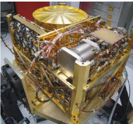
The Sample Analysis at Mars (SAM) instrument inside the Curiosity rover includes a gas chromatograph–mass spectrometer, which analyzes soils collected from the surface. Credit: NASA-GSFC
