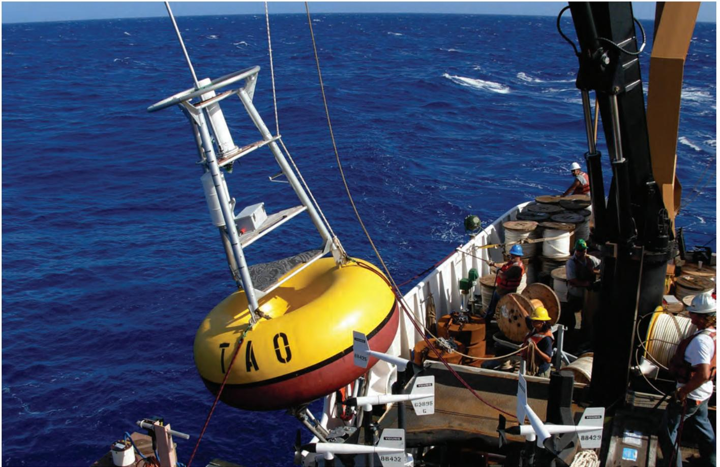
A Tropical Atmosphere Ocean buoy, part of a system collecting temperature, salinity, velocity, and surface meteorological data that inform climate predictions of ENSO, is lowered into the Pacific Ocean near the equator. Credit: Lt. Cdr. Matthew Wingate, NOAA Corps, CC BY 2.0 ([bit.ly/ccby2-0](https://bit.ly/ccby2-0))
