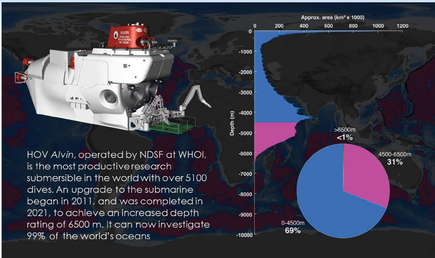
Fig. 1. Roughly 69% of the seafloor was accessible to Alvin before (blue) its recent upgrade was completed. Following the upgrade (magenta), 99% of the seabed is now within the submersible's reach. Credit: Courtesy of S. Adam Soule, ©Woods Hole Oceanographic Institution
