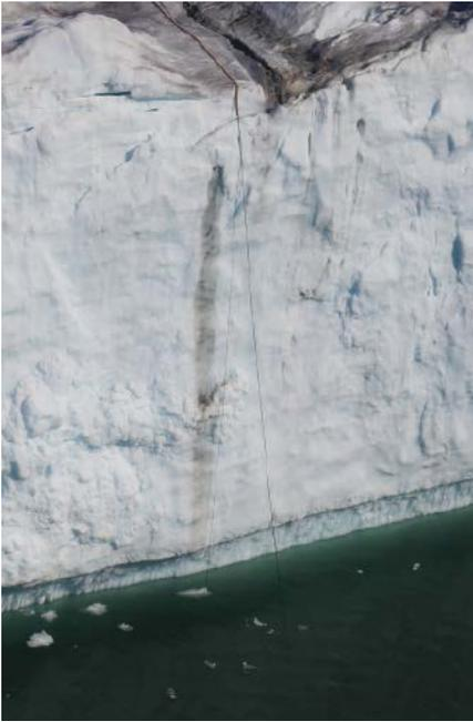
An image taken from a helicopter shows the deep-water sensor cable at the calving front being dragged away from the ice cliff by a strong underwater current created by a subglacial plume. Credit: Shin Sugiyama
