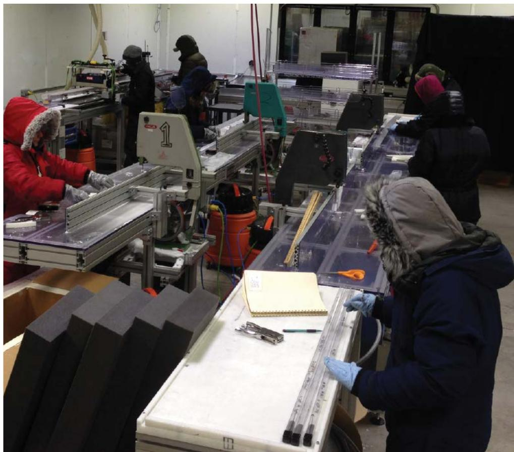
At the National Science Foundation Ice Core Facility, researchers cut samples retrieved from the South Pole Ice Core project to send off to the collaborating universities for analysis. Credit: NSF-Ice Core Facility
