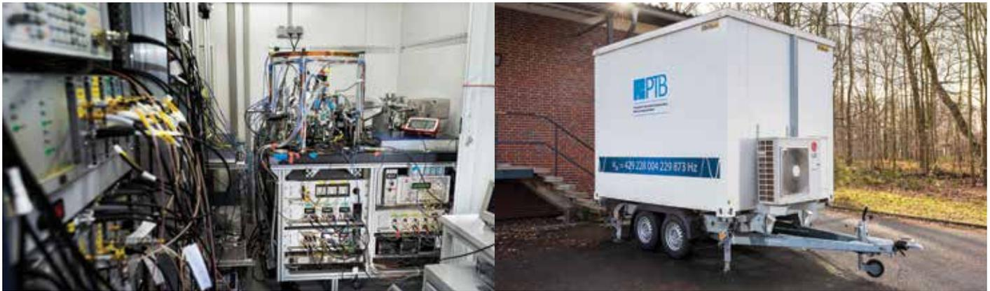
The transportable optical clock of the Physikalisch-Technische Bundesanstalt (PTB), the National Metrology institute of Germany (left) is housed inside a trailer (right).
