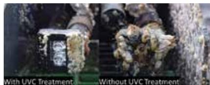
Conductivity data collected using a conductivity probe deployed at sea for several months and treated with UVC light (left) matched very closely with true values, whereas data collected from a biofouled probe not treated with UVC (right) drifted away from the true values within a week [Bueley *et al.*, 2014]. Credit: Ocean Networks Canada and AML Oceanographic
