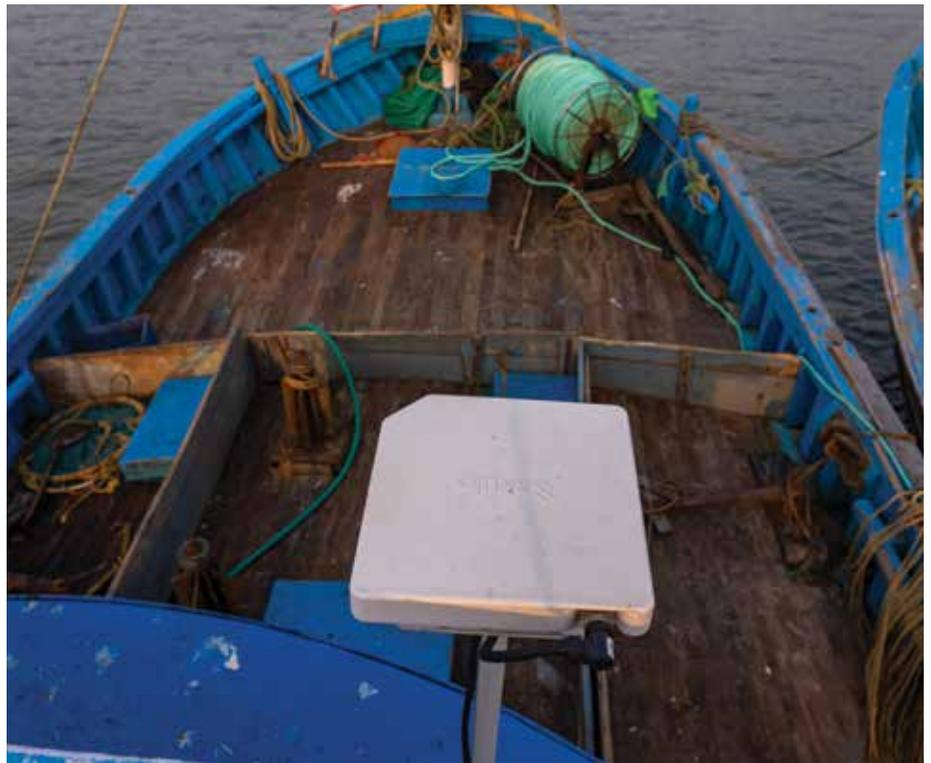
Skylo Hub provides a new way for fisherfolk to communicate safety conditions, fishing zones, and even prices using satellite technology. Credit: Skylo
