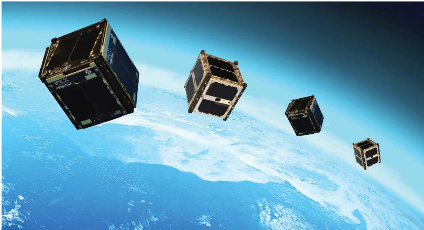
A constellation of CubeSats could help map where atmospheric and tsunami waves are heading before ground-based receivers can detect them. Credit: NASA/JPL-Caltech
