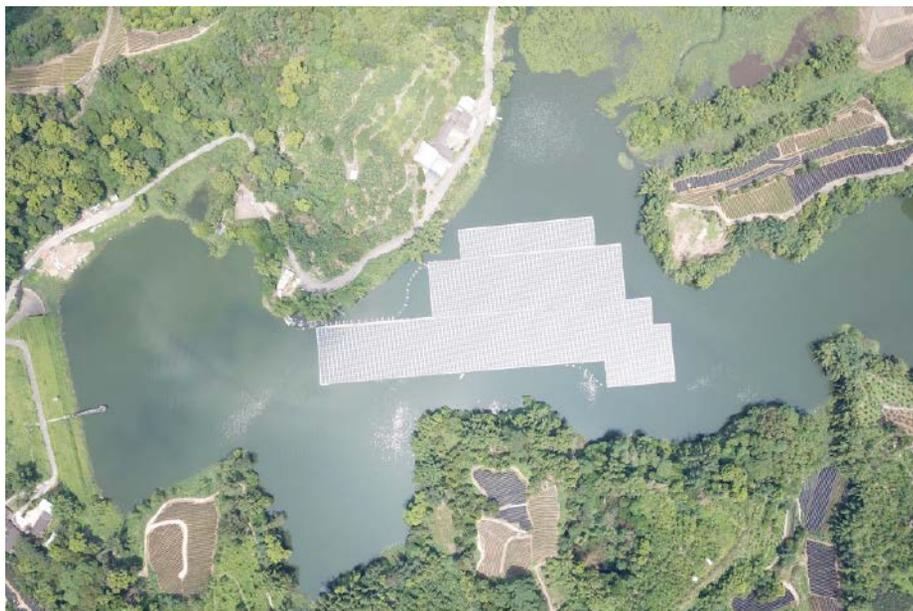
In 2022, a floating solar photovoltaic (floatovoltaic) power generation system with an installed capacity of 1.972 megawatts was installed in the Neipuzi Reservoir, located in Minxiong Township, Taiwan. Credit: Ministry of Economic Affairs Water Conservancy Agency
