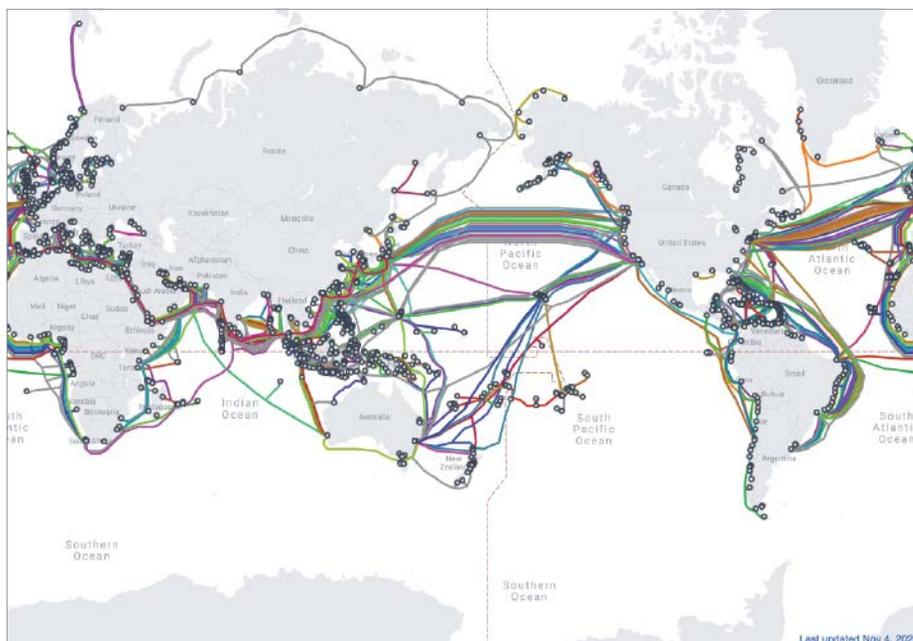
In this map, colored lines depict the locations of subsea cables. They cross oceans and wind their way around continents, stopping at various hubs, shown as open circles, along the way. Credit: TeleGeography’s Submarine Cable Map, CC BY-SA 4.0 ([bit.ly/ccbysa4-0](https://bit.ly/ccbysa4-0))
