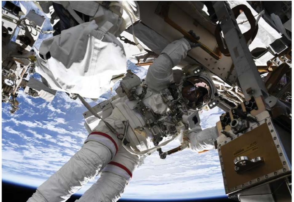
During a 16 May space walk, Drew Feustel installs external wireless antennas and replaces an external light and camera on the International Space Station's truss. Credit: Ricky Arnold/NASA
