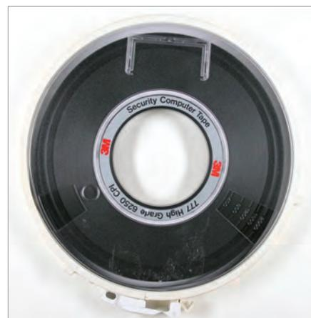
Astronomers once stored telescope data on 9-track tapes. Credit: Hannes Grobe, Wikimedia, CC BY-SA 2.5 ([bit.ly/ccbysa2-5](http://bit.ly/ccbysa2-5))
