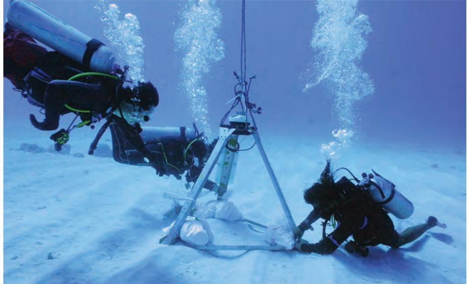
Researchers install sensors on the seafloor to measure ocean currents. Credit: C. E. Marin/Nortek
