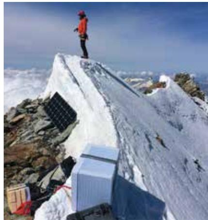
Scientists placed a solar-powered seismometer near the summit of the Matterhorn to record ambient seismic vibration data. Credit: Jan Beutel/ETH Zurich
